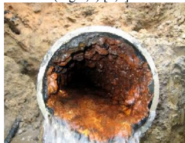
Fig-1: Rusting in a drainage water pipeline
